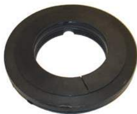
Failed Seal Resulting from Improper Fit
