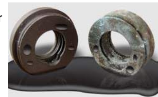
ProTech vs. metallic isolator after soaking 30 days in acid
