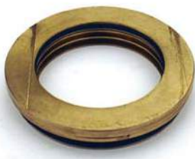
Failed Seal Resulting from Improper Installation
